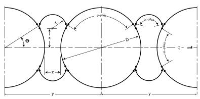
O is measured to the center of the 30° connection
