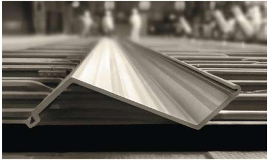
tion, which accounts for less than one percent of the total wall area. AZ sheets are produced with a Larsen interlock and have the lowest rate of conductivity among sections produced. Not only is the potential penetration identified, it is minimized. A non- structural seal weld is applied to every exposed interlock to assure a watertight seal for the life of the structure.
